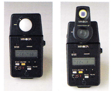
Multi-mode Flash Meter. The multi-mode flash meter has several modes, allowing incident-light, reflected-light, flash, and continuous-light readings. On the left, it is set up for continuous incident-light meter readings. On the right, it is set up for reflected-light flash meter readings, having a 5° reflected-light attachment with viewer in place of the incident dome. This meter can be used for either continuous or flash readings in both incident and reflected modes. In flash metering mode, it will even combine the effect of both flash and continuous light.
