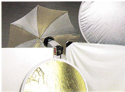
Tools for Diffusion by Reflection. At bottom center and top right are circular cloth reflectors supported by a flexible spring-steel band, which can be coiled for portability. In the middle are a white foamcore board and a white cloth stretched on a plastic pipe frame. At top left is a photographic umbrella.
