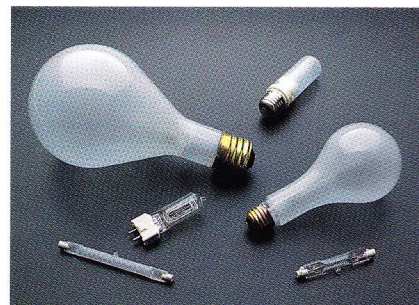
Incandescent Bulbs. At top left is a mogul-base 1000 watt photoflood. At right center is a standard-base 500 watt photoflood. The remainder are variously styled quartz-halogen lamps, ranging in wattage from 600 to 1000.
