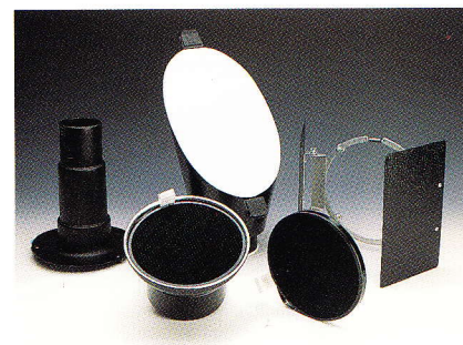
Tools for Restricting Light. All of these tools are designed to be attached to studio lamp housings. From left to right: cylindrical snoot, coarse honeycomb grid in holder, special truncated cone with white interior for lighting backgrounds, fine honeycomb grid, barn doors.
