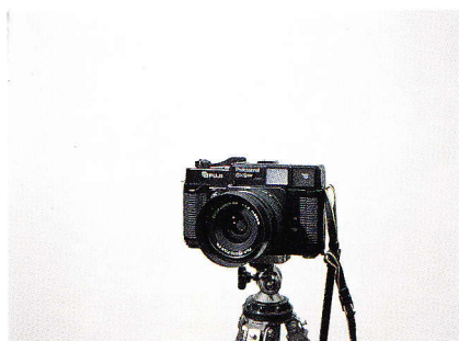
Use of a Gobo to Prevent Lens Flare. A. Without a gobo, light from a studio light falls directly on the lens, as evidenced by the shadow crossing the lens and the specular reflections of the light source seen in the lens surface. Even the use of a lens shade has not prevented flare-producing light from striking the lens.
